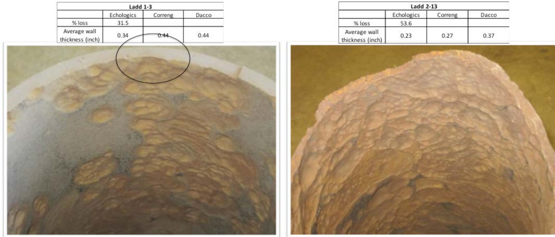
Figure 10: The remaining wall thickness measurements of adjacent pipe segments made using acoustic testing and two forensic analysis. The acoustic test rightly tracked which pipe had a lower remaining wall thickness.
